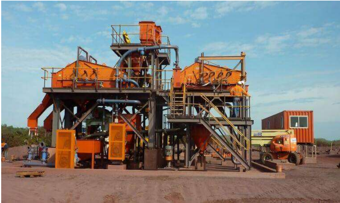
Figure 9: Dense Medium Separation
